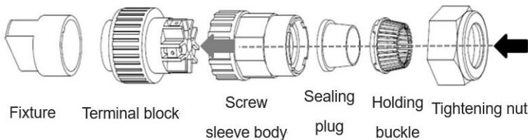
4. Push the holding buckle and the sealing plug into the screw sleeve body, and then assemble the terminal block, the screw sleeve body and the tightening nut together. First clamp the terminal block with a plastic clamp, then screw the screw sleeve body onto the terminal block, and finally tighten the tightening nut.
