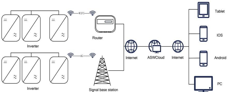
Method 1 only one inverter with the 4G/WiFi Stick, the other inverter be connected through the RS 485 cable.
