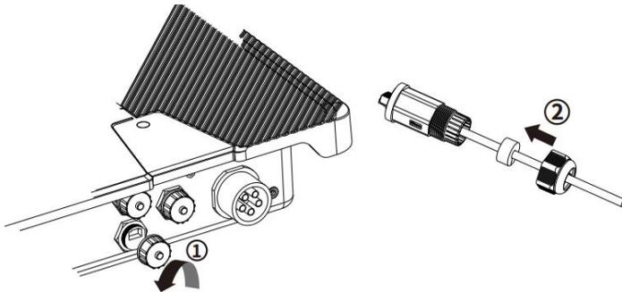
3. Insert the cable into the corresponding communication connector in the order of the arrow, tighten the sleeve and the forcing head screw at the tail.
